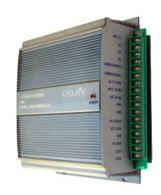
Powerful logic circuits and algorithms are used in the microprocessors that constitute the heart of the solid state controller. The proprietary firmware utilizes multiple sensor inputs and processes them for real time, continuous and precise gas flow control. The circuits have extensive fault detection and autonomous fault correction subroutines.
