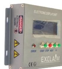
The proprietary dual fuel algorithms uploaded in the onboard firmware are designed to operate the engine at the **maximum possible gas substitution** based upon dynamic, real-time engine performance data being constantly correlated with threshold values and safety parameters and customized to engine make, model, output, etc.
